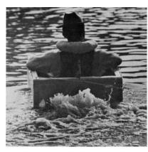
The design limitations disallowed gasoline engines. This student used an auto starter with a battery as his propulsion. He is sailing along here at 6 m.p.h.
